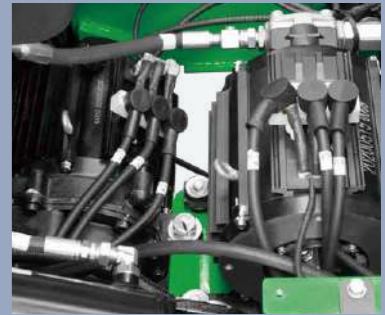
Both the traction and oil pump adopt permanent magnet synchronous motors for the Enpower controller
